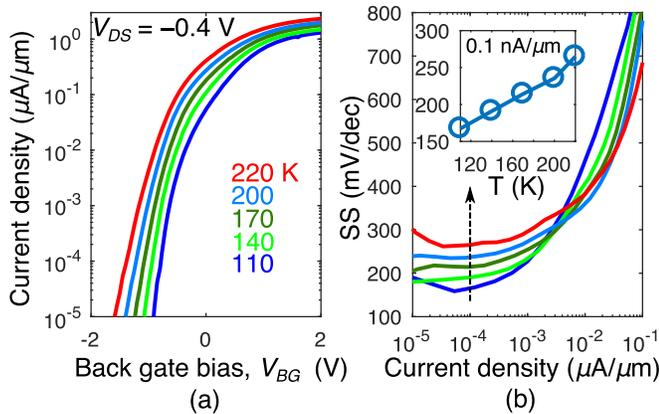
Fig. 4. (a) Temperature dependence of the back-gate transfer characteristic and (b) subthreshold swing for  $V_{DS} = -0.4$  V. The inset shows the SS temperature dependence at a  $10 \text{ nA}/\mu\text{m}$  drain current density.
