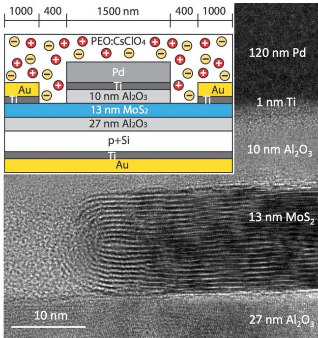
Fig. 1. Nanoribbon MoS<sub>2</sub> transistor cross-sectional schematic and transmission electron micrograph (TEM) along the 700-nm width. This TEM was made on completion of the measurements discussed in this paper.
